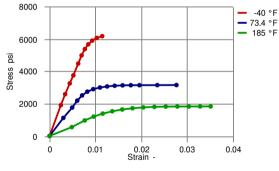
No yield at -40 °C 23 °C yield at 0.01775 strain, 21.608 stress 85 °C yield at 0.02791 strain, 12.546 stress
