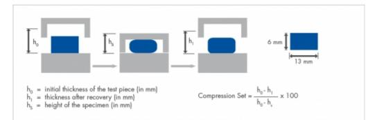
The specimen is compressed by 25%. The compressed specimen is heated to the test temperature. DIN ISO 815 discribes two methods.
