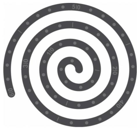
Test conditions: 760 bar (specific pressure) / 200 °C Flow Spiral Dimensions 2 mm x 5 mm
