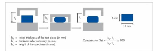
The specimen is compressed by 25%. The compressed specimen is heated to the test temperature. DIN ISO 815 discribes two methods.
